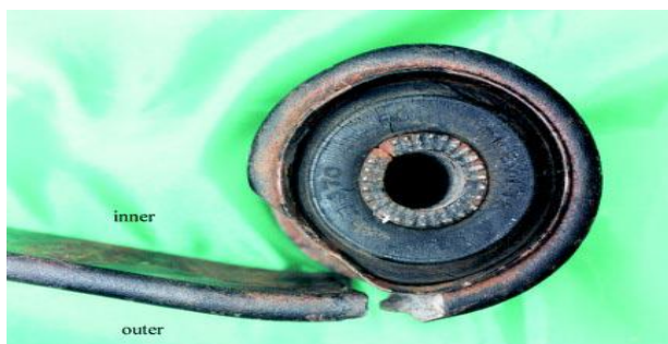
Fig.4 Eye end failure
